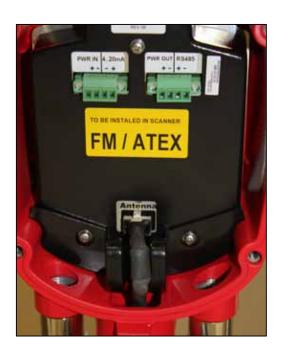
2. Inside the enclosure, you will disconnect the 10-pin connector from the electronic card and pull out the cable strain relief.
