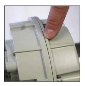
18. Now it is important to note the placement of the lead transducer. There are two markings that are used to identify the lead transducer, one is on the widest part of the transducer body in the form of a raised line, and the other is a notch just above the threads on the neck of the transducer.
