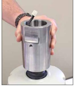
7. It simply screws onto the neck of the scanner. Snug the adapter to the transducer using a 24-inch pipe wrench.
