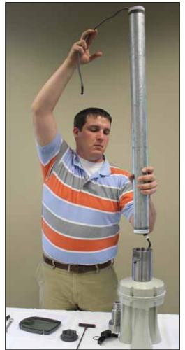
12. The next step is to fish the cable through the extension pipe.
