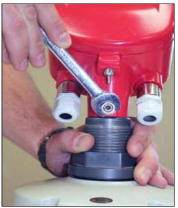
23. Tighten the hex set screw with a 5/32" allen wrench and secure the lock nut with a ½-inch wrench.
