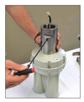
9. Then take the extension cable and hook it up so the locking mechanism connects, making sure the locking tab connects.
